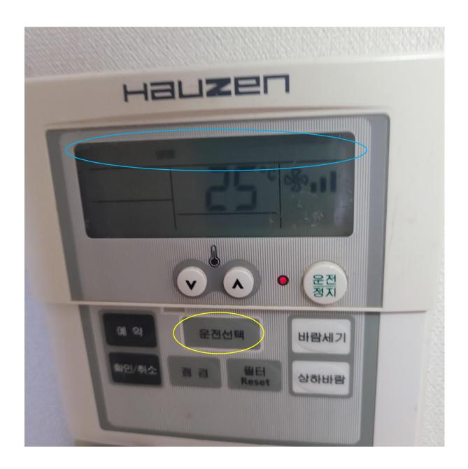
And finally, we have cycled back to "냉방." This word means, "cooling." This is the option you are looking for after getting back to your dorm room on a hot day. Something to note is that the encircled button is the only one that I have pressed, but, as you may have noticed, the settings on the other boxes (aside from the top row) have been changing as well. Not important. We can ignore that.
