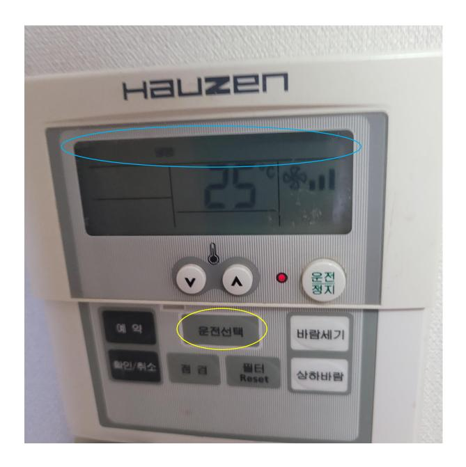
This is what mine (the one in my room) looks like when I turn it on. And this is the optimal setting for producing the coolest air. To achieve this, we must cycle through the different modes of the air-conditioning unit. Let's start with the encircled "운전선택" button. Look at the top row (the area inside the blue circle) on the screen and compare this picture with the following other pictures.
